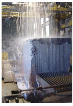
Above. In the quarry, two Benetti wire saws cut the stone from the face 1,000 tonnes at a time while seven more Benettis trim the blocks on the quarry floor. You can watch a block falling on YouTube.
