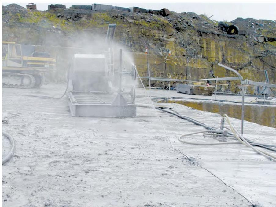
Above. In the quarry, two Benetti wire saws cut the stone from the face 1,000 tonnes at a time while seven more Benettis trim the blocks on the quarry floor. You can watch a block falling on YouTube.
